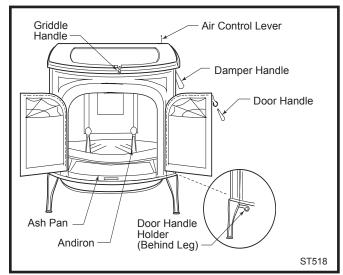
Fig. 18 The Intrepid II controls.
